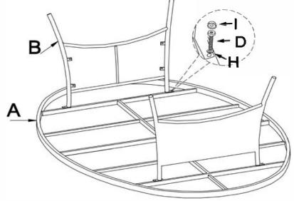
Step 1. The table top is placed facing down on a soft surface, Attached the legs panel (x 2) to the table top.
