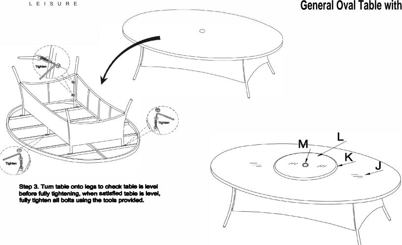
Step 4. Finally place the glass plate onto the table top, Place the lazy Susan onto the table lining up the holes for the parasol, slide the parasol protector ring through the centre holes of the table and attach the back nut from the underside of the table. Do not over tighten as this will prevent the Lazy Susan from turning.
