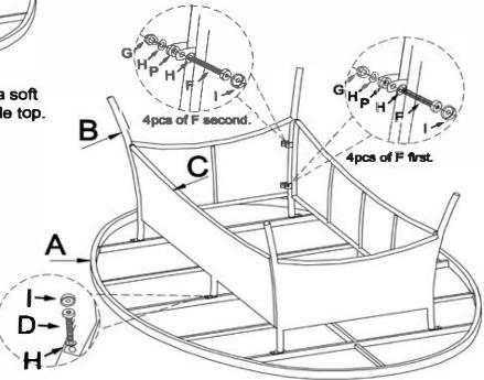
Step 2. Attached the Side Panels to the leg panels.
